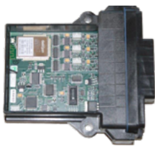
The NaviLink gateway controller designed and manufactured in partnership with Dorigo Systems.
